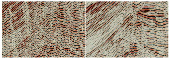
MF technology was applied to low-fold and low-quality data from northwestern Russia (Timano-Pechora Basin). An interpreter would have a very difficult time unraveling this complex geological history using the conventionally processed section on the left. In the MF section on the right, the picture is much clearer. (Images courtesy of Geomage)
