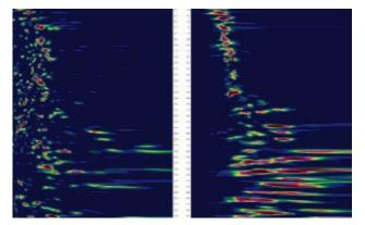
A velocity analysis of the original data also was included in the proposed data enhancement idea (left). The velocity analysis improves with the MF-enhanced data (right).
