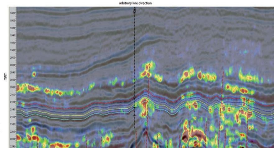
**Figure 3** Arbitrary line showing the PSTM data in the background with migrated diffractivity in colour. The interpreted horizons show the top, inter-formation and base of the Bazhenov.
