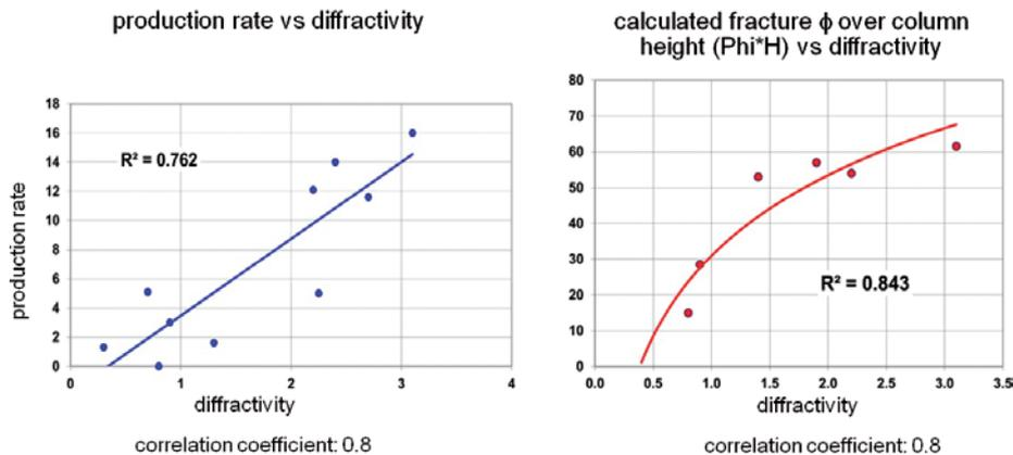
Figure 4 Left site: normalized production rate versus average diffractivity. Right site: calculated fracture porosity multiplied by the column height versus average diffractivity.
