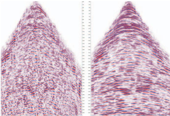
An original CMP gather was part of the proposed data enhancement idea. The original common supergather (left) has low signal-to-noise ratio and is characterized by a complex kinematics of reflection events due to the surface topography and subsurface geology. The MF-enhanced gather (right) shows essential signal-to-noise improvement, and it preserves all main kinematic and dynamic features of the original data.
